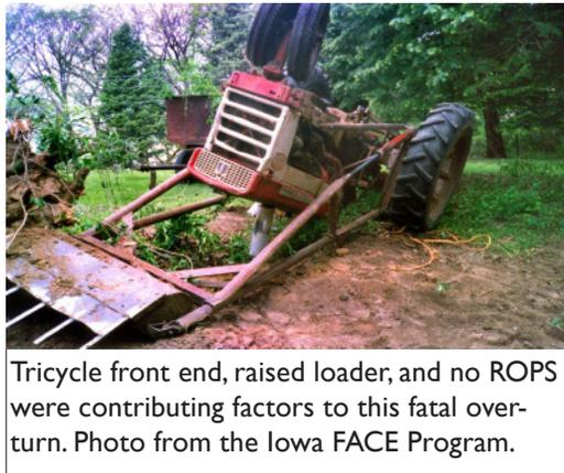
Tricycle front end, raised loader, and no ROPS were contributing factors to this fatal overturn. Photo from the Iowa FACE Program.
