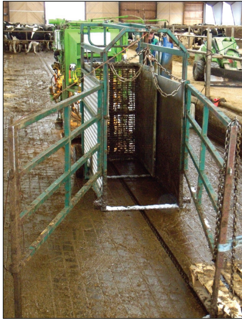
Figure 2. Mobile single-file alley and trimming chute placed in a scrape alley (photo: Cecilia Lindahl).
