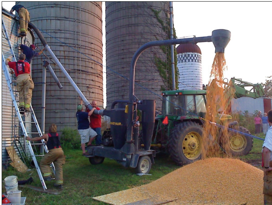
Figure 6. A grain vacuum used in an attempt to rescue a man entrapped in a bin on an Indiana farm.
