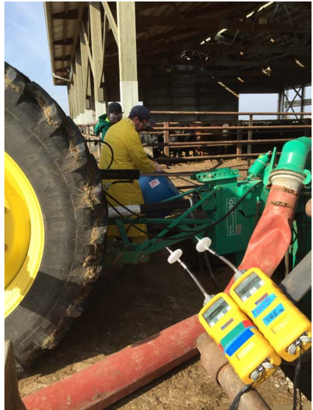
Figure 3: Manure gas monitoring during cattle manure pumping field response.
