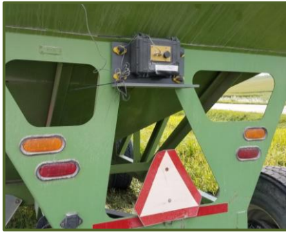
Figure 4: Rugged case containing camera, GPS, and power supply mounted to the rear of a grain wagon
