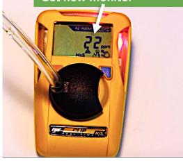
Aerosol bump test may not reach target concentration (25 ppm) using the aerosol spray method
