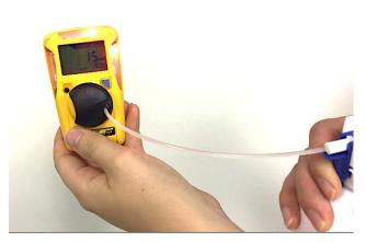
Aerosol bump test may not reach target concentration (25 ppm) using the aerosol spray method
