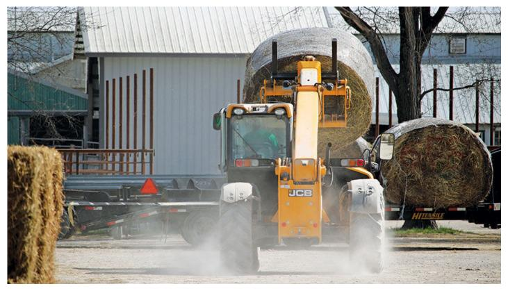
An enclosed operator compartment and an attachment designed to hold bales improve bale handling safety. Photo by Stephanie Leonard
