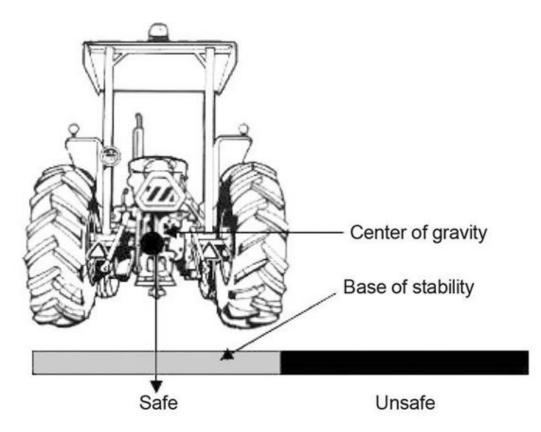
Tractor rollovers occur when the tractor's center of gravity moves outside of the base of stability. Image courtesy the National Ag Safety Database
