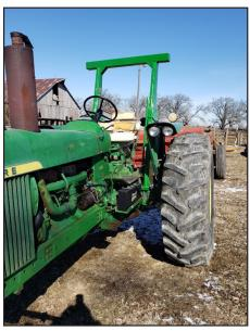
A 1968 John Deere 4020 tractor in Scott County, Iowa after ROPS installation.
