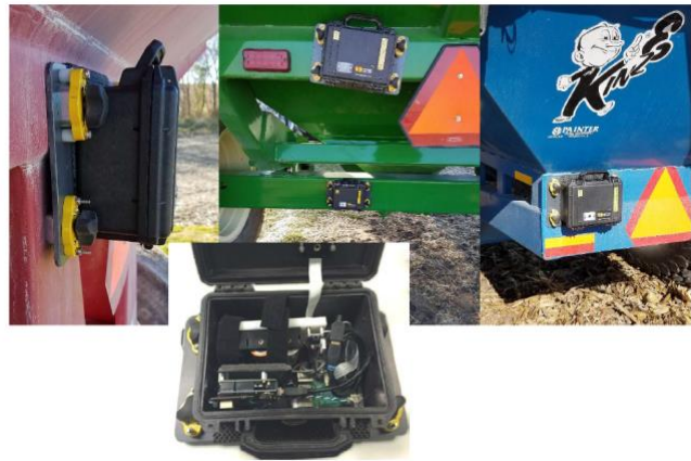
Figure 2: Mounted SaferTrek devices in weather-tight boxes.
