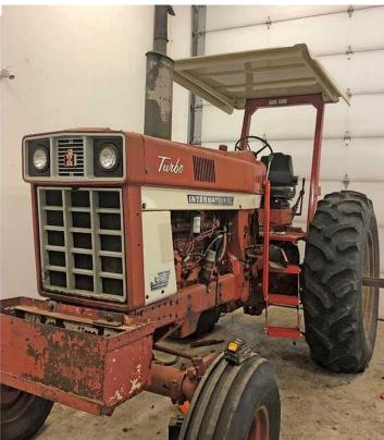
An International 1466 tractor in Plymouth County, Iowa, before and after ROPS installation. In addition to the ROPS, the owner added a canopy and steps with a hand rail. Photos courtesy I-CASH
