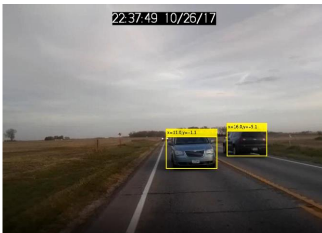
Figure 8: Screenshot from video processing, identifying following and opposing vehicles and their respective distance from the farm equipment (camera mounted on farm vehicle, rear-facing).
