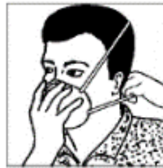
Position respirator under chin with nose piece up. First, pull top strap over head, then bottom strap
