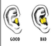
4) HOLD plug in place as it expands to ensure proper fit
