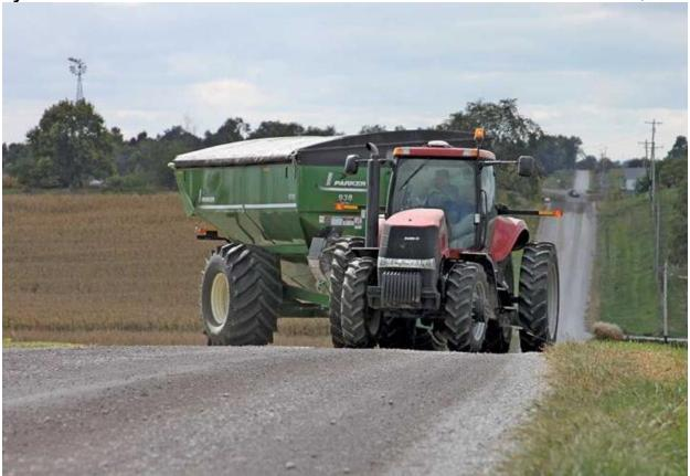
Flashing amber lights and reflective tape help define the size and shape of farm equipment, which helps other drivers safely navigate around you.
