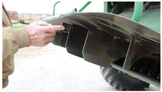
Some close calls don't make the news, like how a sharp piece of loosened steel at the combine discharge tore a sleeve and could have torn flesh.
