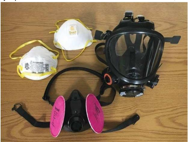
Air-purifying respirators include: N95 filtering facepieces (upper left); half-face respirator with P100 filters (bottom); full-face respirator without cartridges or filters (right).
