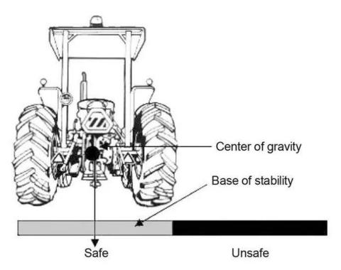
Tractor rollovers occur when the tractor's center of gravity moves outside of the base of stability. Image courtesy the National Ag Safety Database
