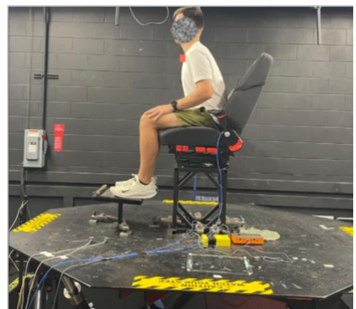
Figure 10: Illustration of exposure measurement validation involving human subjects seated on agricultural machine seat mounted to a human-rated motion platform.
