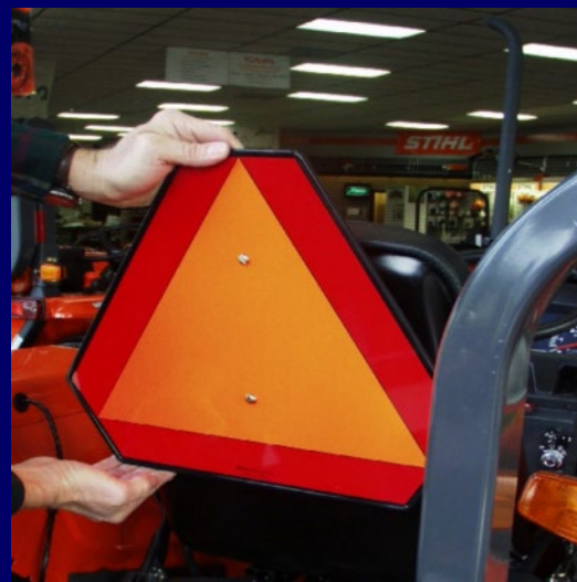
Figure 4.14.f. SMV emblems are required on vehicles designed to travel less than 25 mph while occupying public roadways. SMV emblems should be visible from no less than 1000 feet to the rear of the tractor or towed implement. Therefore, mounting height may vary from 2 to 10 feet above the road surface. Replace faded, damaged SMV emblems.
