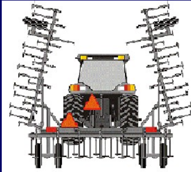
Figure 4.14.b. Lighting and marking standards may or may not be the standards for your state. Check your state laws.
