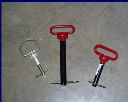
Figure 4.14.d. Secure hitch pins with locking clips as shown.
