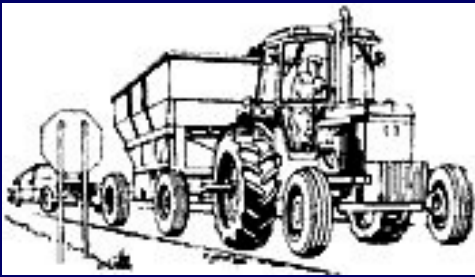
Figure 4.14.g. A best practice for transporting wide loads on a public roadway is to use an escort vehicle to assist in alerting other motorists. Be a courteous tractor operator to bring good public relations to the farm community.
