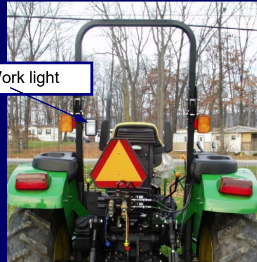
Figure 4.14.c. Be sure that a work light that points to the rear is off during road travel at night. Single white lights may not be recognized as slow-moving or as a tractor light. Also if SMV emblems are worn or obsolete, replace them with newer more reflective SMV emblems.
