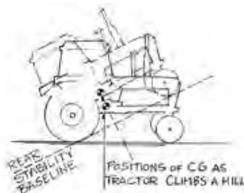
Figure 4.12.f. When a tractor is pointed up a slope, the CG is closer to the rear stability baseline. Illustration by Jeff Mathison
