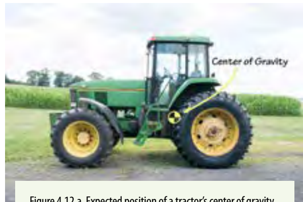
Figure 4.12.a. Expected position of a tractor's center of gravity. Credit: Jeff Mathison
